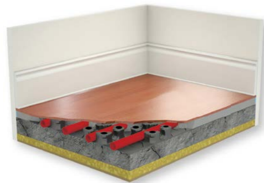
MICROPLATE WITH INSULATION BELOW SLAB
