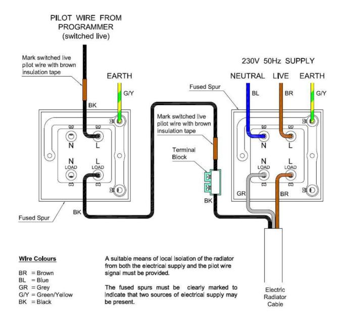
PLEASE NOTE: THE TOUCH4 IS A PROGRAMMER ONLY. TO CONTROL THE TEMPERATURE OF THE ELECTRIC DÉCOR AND COLUMN RADIATORS, THE SUPPLIED RF THERMOSTAT MUST BE USED. PLEASE REFER TO THE ELECTRIC DÉCOR, ELECTRIC COLUMN AND TOUCH4 INSTALLATION INSTRUCTIONS FOR MORE INFORMATION
